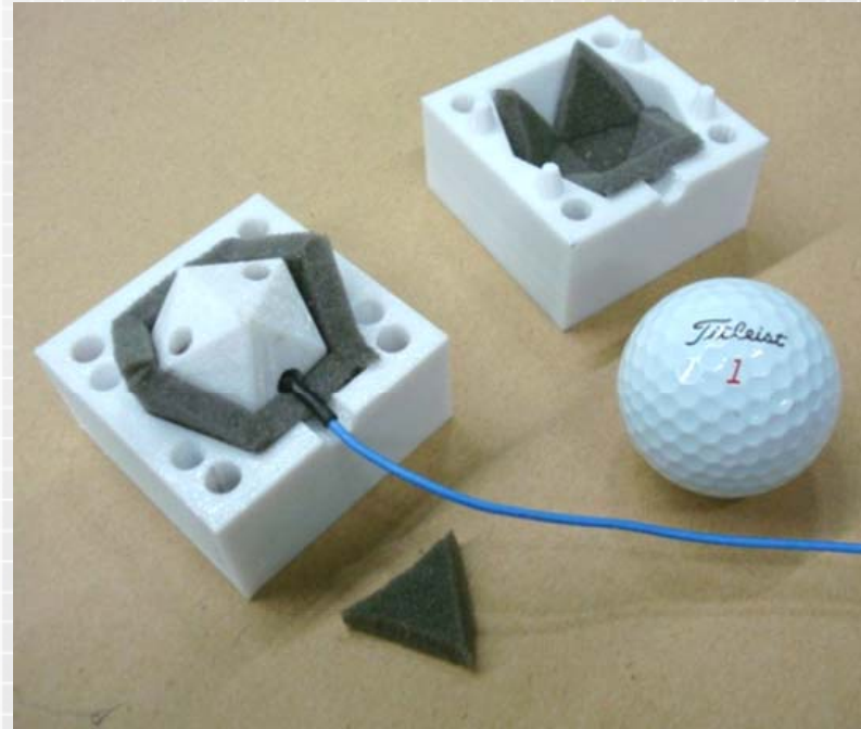
Icosahedron mount for tri-axial accelerometer
