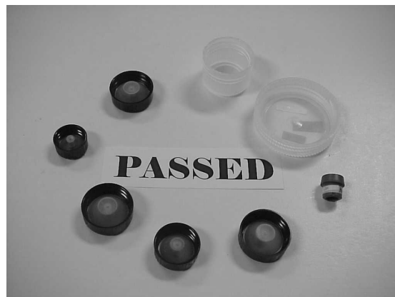
Figure 3: Closures that showed no leaks after tests
