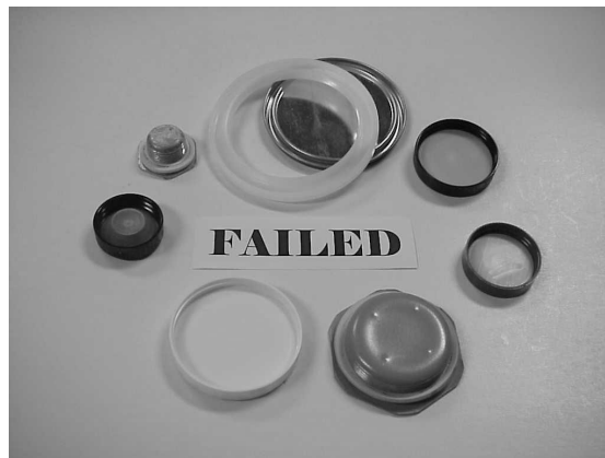
Figure 2: Closures that showed leaks after tests
